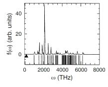
Vibrational density of states of a electronic system (continuous spectra) as compared to a harmonic approximation (stick spectra) and the highest frequency phonon mode (triangle). Here states are well separated.
